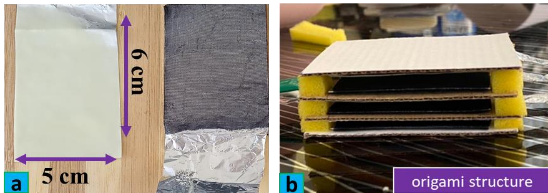
Figure 1. a) description of nylon and PU materials b) description of TENG with origami structure
