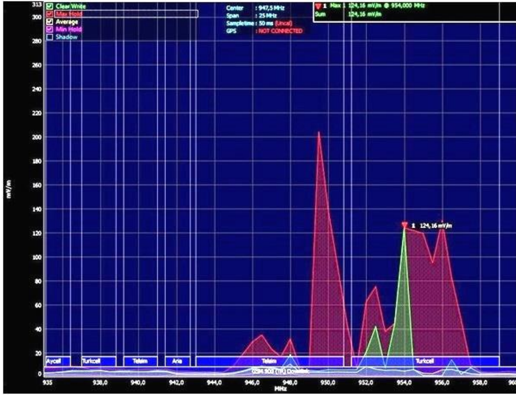
Figure 2. A typical spectrum of the electric field strength measured at GSM 900 MHz frequency by using a Spectran HF 60105 V4 portable spectrum analyzer and a laptop loaded with MCS software.
